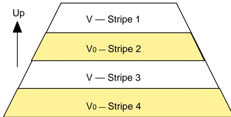
**Figure 1** Arrangement of voltage stripes for the outer sector. The voltage of the shaded stripes  $V_0$  was held constant while the other stripes were varied.
