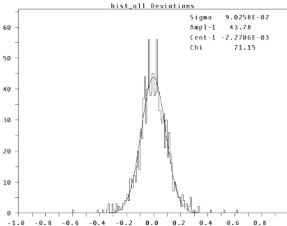
**Figure 5** Difference between expected hit of pad and measured position of the pad. This distribution is for the 4/3 gain data. The units of this plot are in cm.
