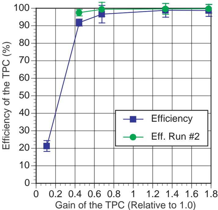
**Figure 4 Measurement of the efficiency of the TPC. Run #2 refers to a reanalysis that was done about a month later.**
