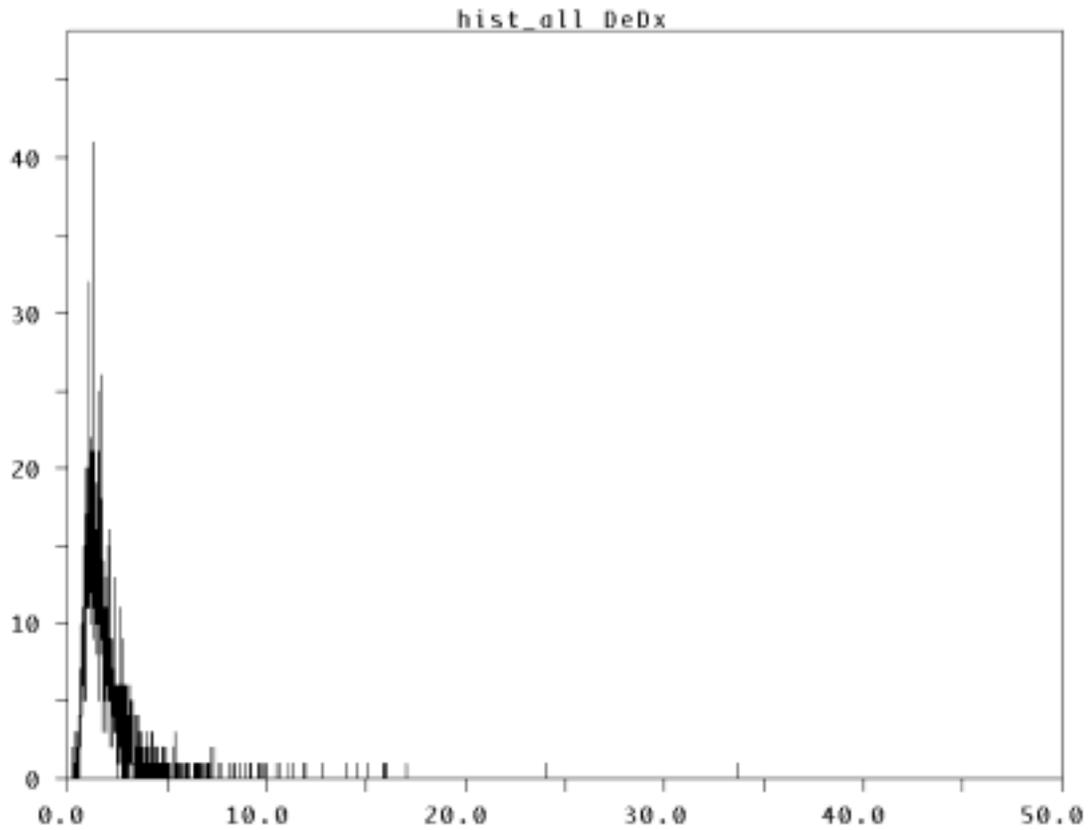
Figure 7 dEdx distribution for the 4/9 gain run. The sum of all of the energy for each pad is plotted.
