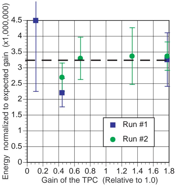
**Figure 8** This plot shows the normalized gain for each of the different runs. The runs refer to the two different passes in the STAR analysis. The dotted line at 3.1 is only to guide the eye.
