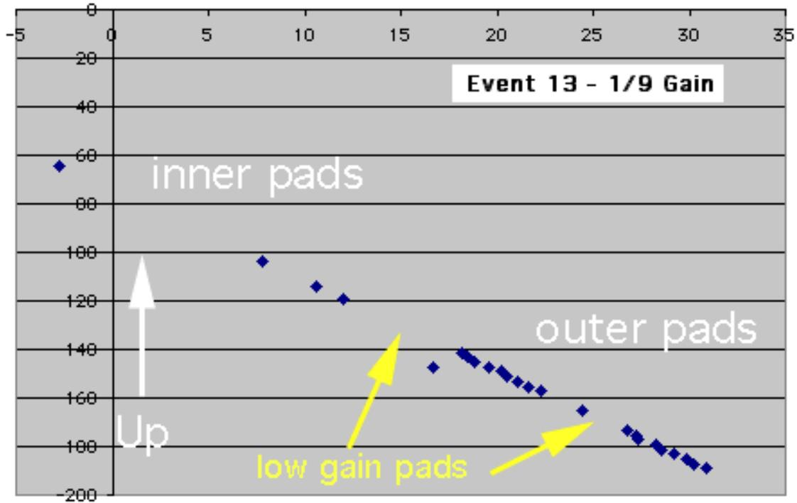
**Figure 2 Plot of the x-y projection of a cosmic ray trigger. This event had a gain of 1/9. The units of this plot are in cm.**
