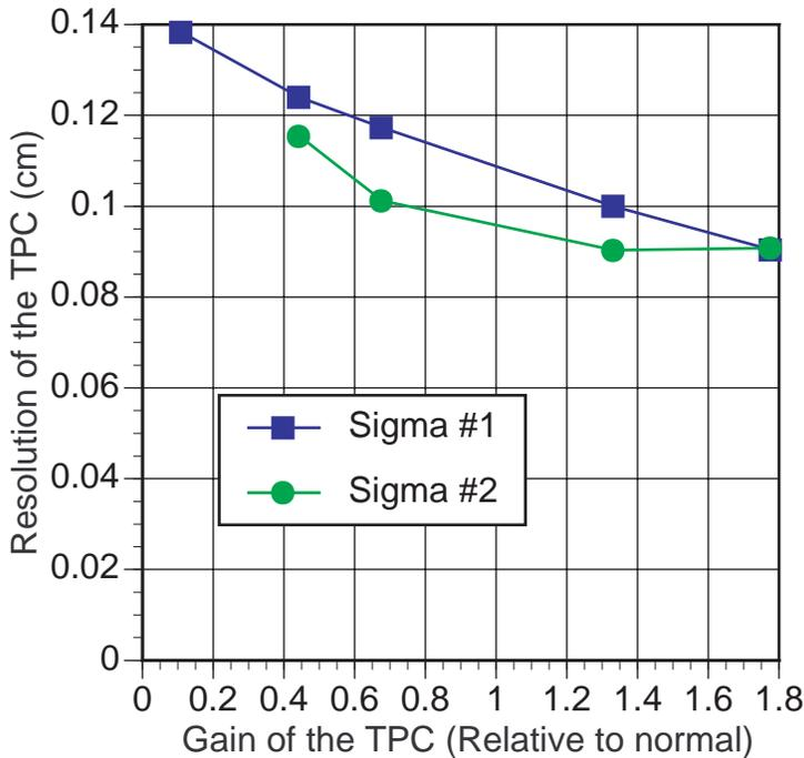
**Figure 6 Measurement of the resolution of the TPC. The number for each data set refers to the analysis number.**
