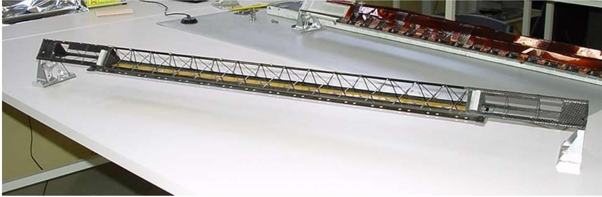
Figure 7 : a carbon fiber mechanical structure of a ladder
