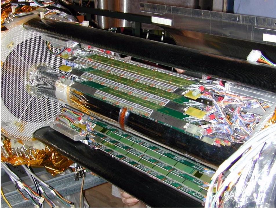
Fig. 6. The final SVT just before installation of the second half-shell installation into the TPC.
