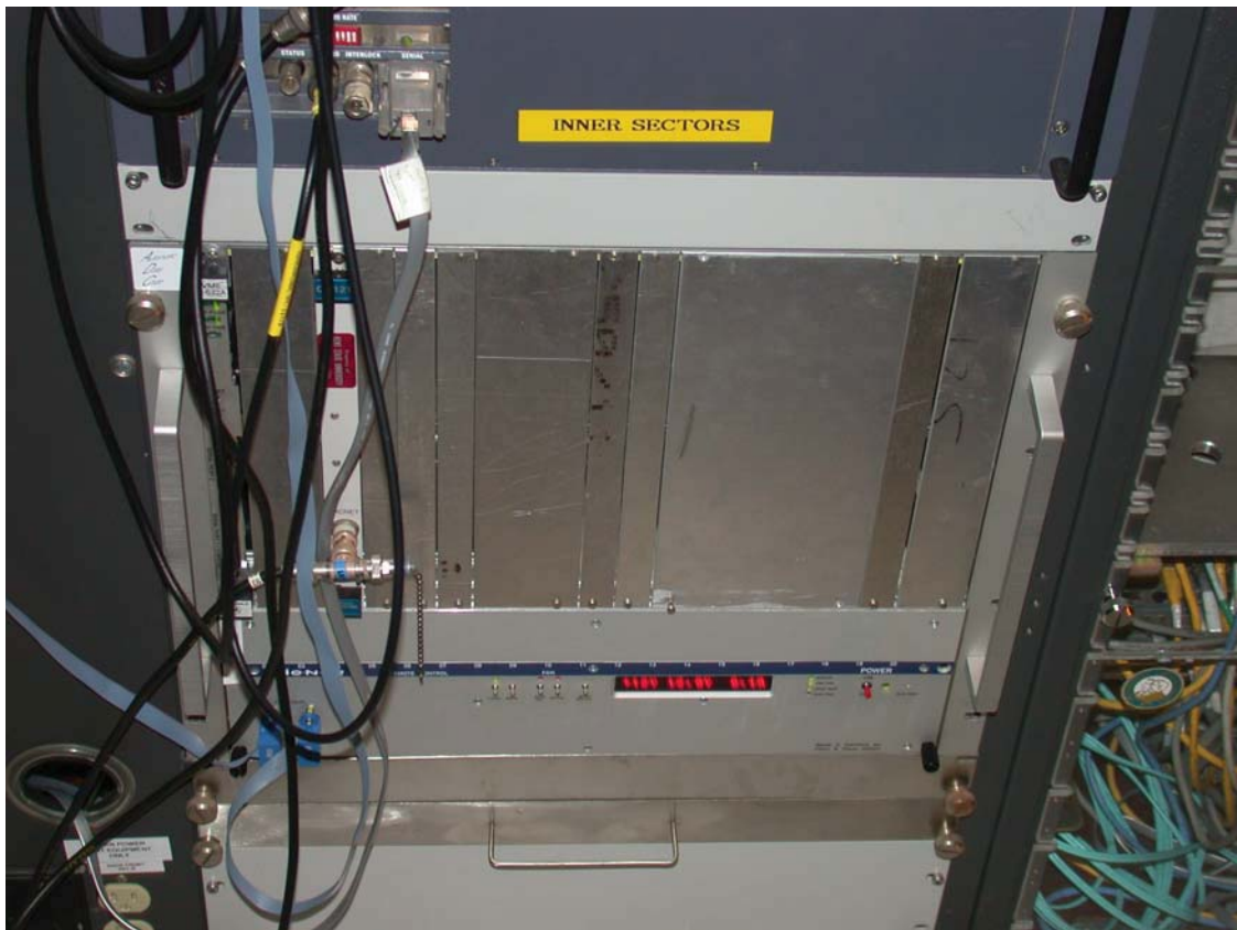
Inner anode VME crate – processor in left slot, also showing ARCNET card. Inner Lecroy is just above the crate.
