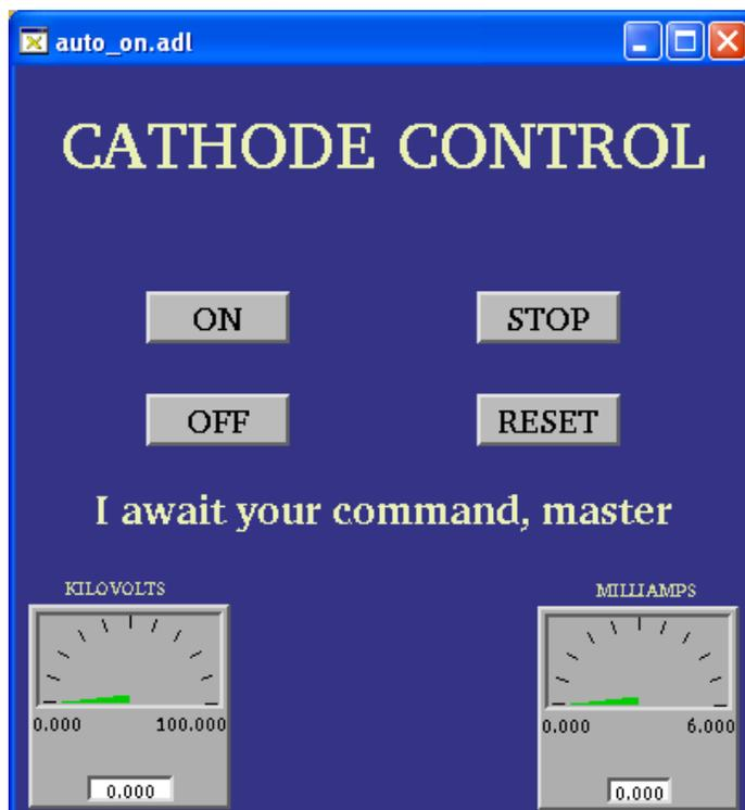
The autoramp program ramps the HV to 10 kV, checks the four field cage currents, then ramps to 20 kV, checks the currents, and then ramps to 28 kV and checks the currents one more time. If the currents are all equal, within specs, the cathode is declared ready for physics.
