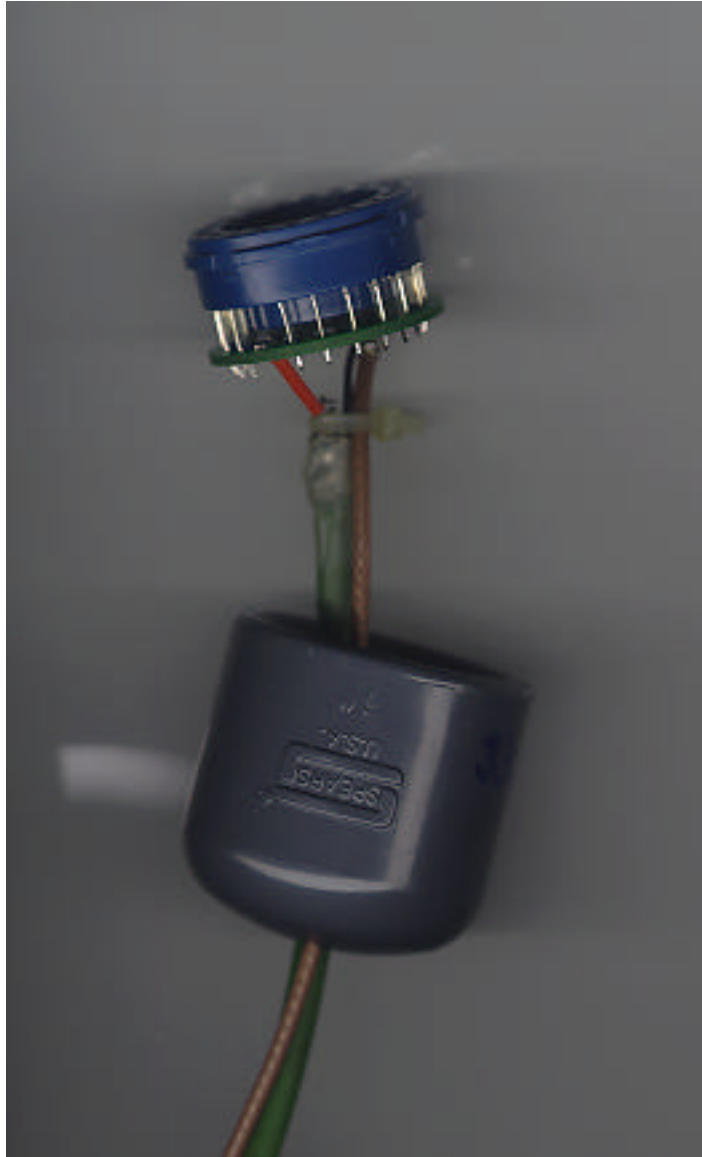
Figure 2: Picture of disassembled base showing printed circuit board soldered to PMT socket and PVC pipe cap housing
