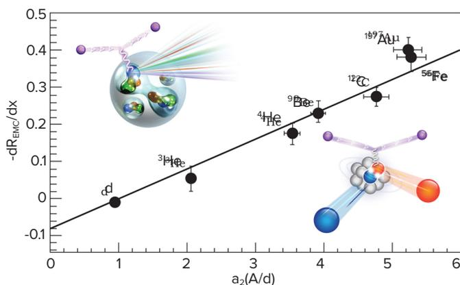
**Figure 2.8:** This plot illustrates, for a sample of eight nuclei, the apparent linear relationship between a parameter that characterizes the number of two-nucleon correlated pairs,  $a_2(A/d)$ , and the strength (i.e., the slope) of the EMC effect. A clear correlation is evidenced by the straight line that all eight nuclei fall on.
