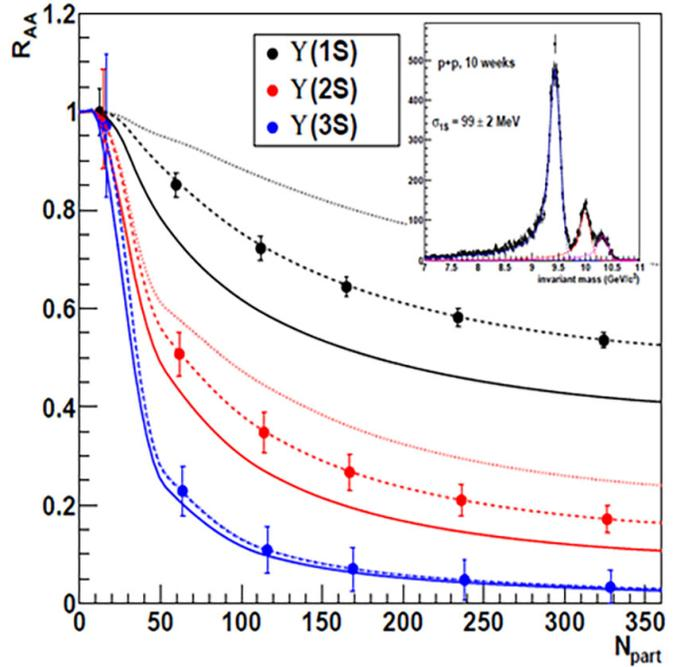
*Figure 2.11: The projected sPHENIX mass separation of the three upsilon states (in the inset) and the projected accuracy of measuring their nuclear suppression in collisions with varying impact parameters. Three sets of theory curves show the melting dependence on the degree of fluid perfection.*
