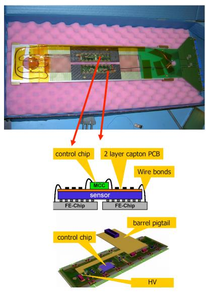
2 Planes with different geometry using ATLAS pixel modules built and operated in NA60 2004 proton run
