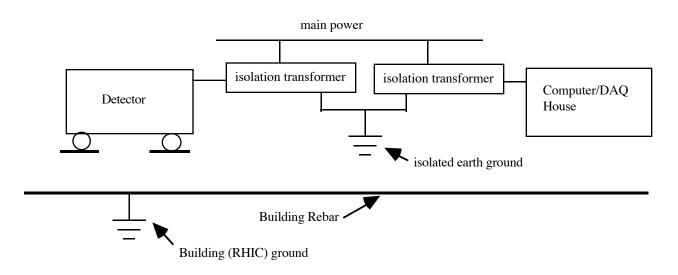
We are using the detector platform and the magnetic iron as electromagnetic shields from the building rebar which we assume will be in contact with RHIC ground. To implement the grounding plan, we need to make the following requirements:
