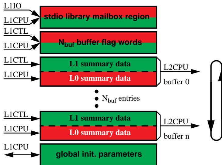
The trigger controller will not perform any reformatting of the trigger data. Therefore the data posted in the L1/L2 input buffers (L0 summary data and DSM input buffers) will be a direct copy of the appropriate memory regions identifying the data format of these buffers. The format of the L1/L2 result fields, however, depends on the analysis code and is outside the scope of this document.
