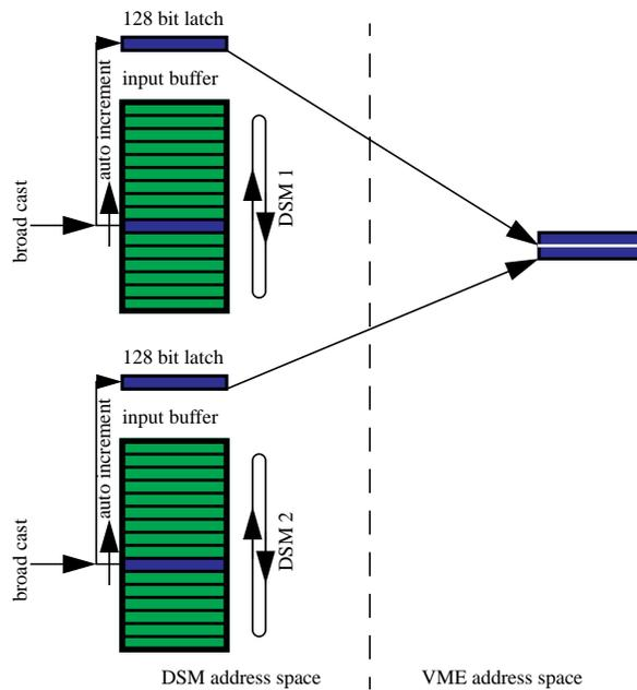
It is therefore possible to program the address decode logic of all DSM boards in one crate to form a contiguous memory space that could be readout with one DMA block transfer. The fact that this memory region is spread out over several VME boards does not matter for the reading DMA engine.
