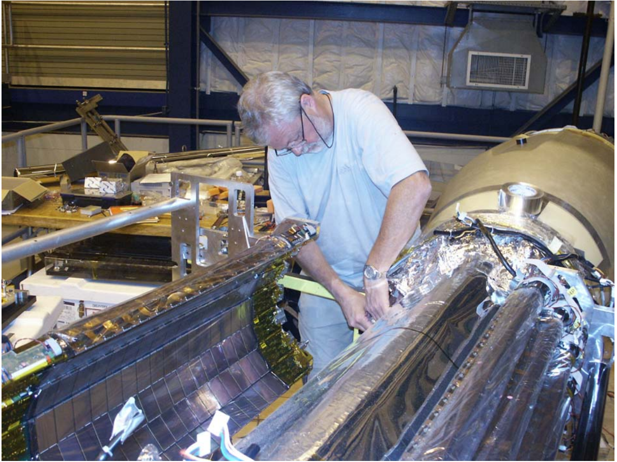
Fig.11: north sector on the rail equipped with its handling tool before installation on the cone (identical for the south sector)
