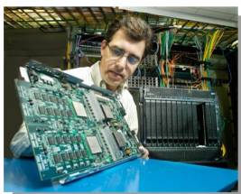
blade11bc4 @IBM, Böblingen: 2 Cell Broadband Engines with 256 kB Local Store at 2.4 GHz
