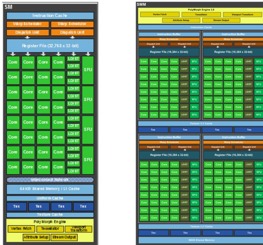
Figure 3.6: Structure of streaming multiprocessors of the Nvidia GTX 480 GPU based on the Fermi architecture (left) [50] and the Nvidia GTX 980 GPU based on the Maxwell architecture (right) [51].
