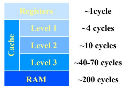
Figure 3.2: Typical access speed to different memory layers on modern CPUs.
